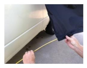
7. Attach the side curtain magnets along both ends of the curtain to the side of the van.
