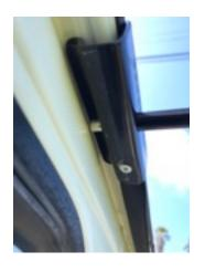
5. Hold onto the right rain gutter bracket firmly (to hold it in place) and insert the other end of the aluminum pole into the hole.
