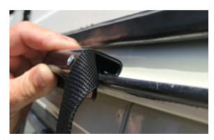
2. Adjust the left rain gutter mount so that it lines up with the body seam between the 2 windows.
