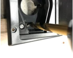
14. Unscrew rubber cap from button and push through the hole in the city water box. Screw rubber cap back on from the front side of the box.
