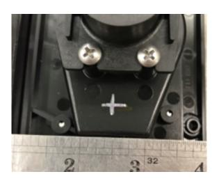
12. Center punch with a scratch awl and drill a 1/8 inch pilot hole. Drill slowly with little
