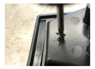
13. Drill a 3/8 inch inch hole from the top into a piece of wood on the opposite side. Drill slowly.
