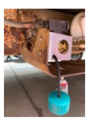
3. Add teflon tape to the 1/2 mpt 90 deg to 3/8 barb fitting and tighten with wrenches until secure.
