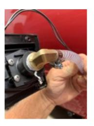
17. Go to the inside of the van and disconnect the city water line from the faucet under the sink.. If you will be using the stock faucet you will have to cap the city water connection on the faucet. If you have already installed a shurflo faucet with the 3 way city water diverter, then disconnect it completely and connect the sink hose from the 3 way valve to the faucet
