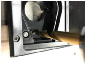
15. Wrap brass 90 deg. fitting with teflon tape and screw into back of gowesty box. Be careful not to cross thread into the plastic box
